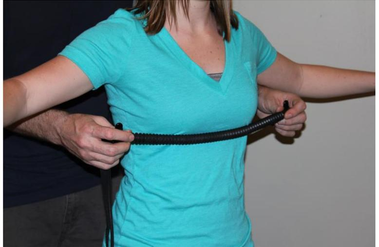
**Figure 2: Attach chest expansion bellows over the rib cage at the location of greatest expansion.**
